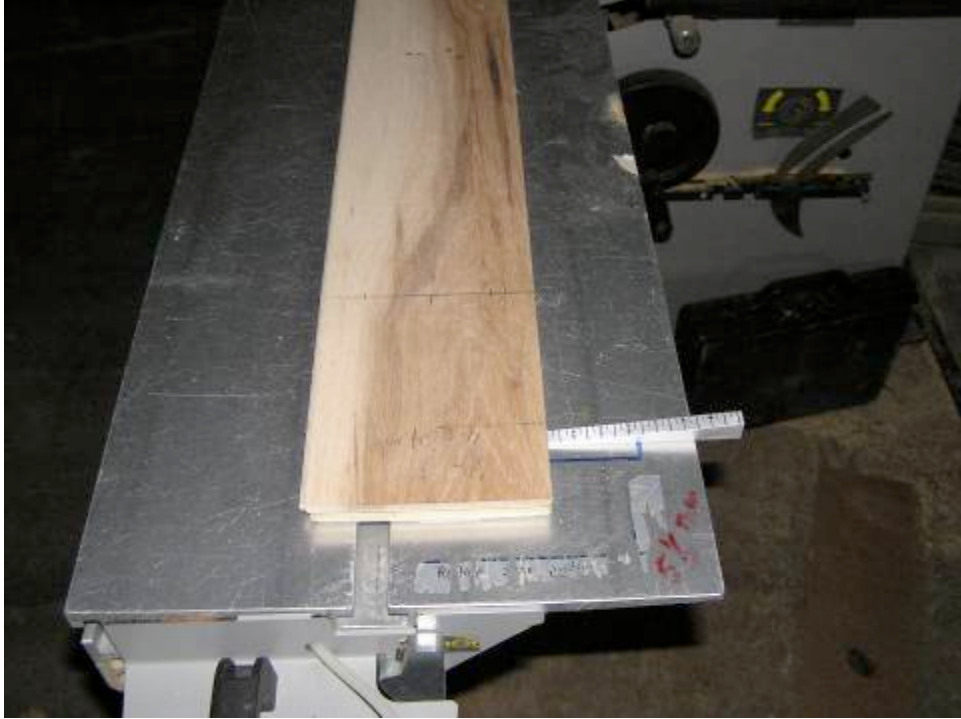
3.--Twist measurement device.
