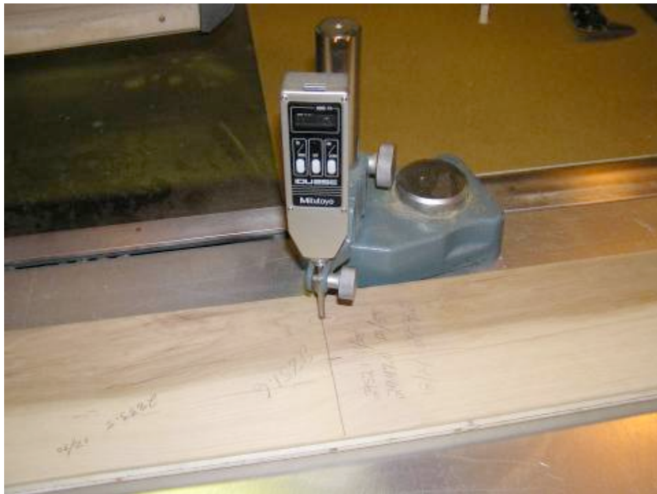
2.--Thickness measuring device and bow/ski measuring device.
