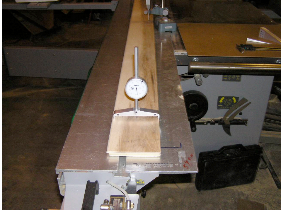
1.--Cup/crown measuring device.
