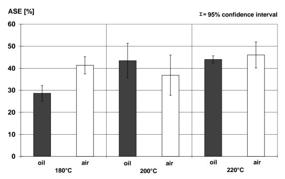
Fig. 5. ASE between 0 and 35% relative humidity of treated Pinus sylvestris L. (10x20x20 mm<sup>3</sup>), n=4
