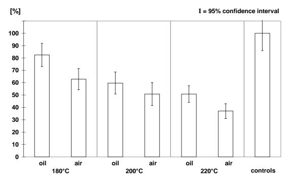
Fig. 4. Changes of the impact bending strength at *Pinus sylvestris* L. (150x10x10 mm<sup>3</sup>) after treatment compared to untreated controls; n=15
