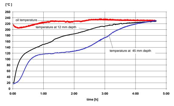
Fig. 2. Course of temperature in the oil and wood during the phase of heating up. *Picea abies* L. Karst., with a cross section: 90 x 90 mm<sup>2</sup>.
