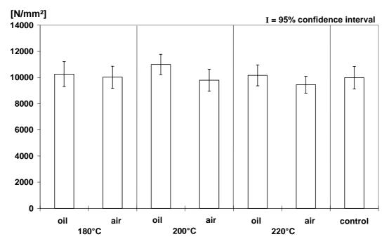
Fig. 3. Modulus of elasticity of *Pinus sylvestris* L. parallel to the fibres (150x10x10 mm<sup>3</sup>) after treatment; n=15
