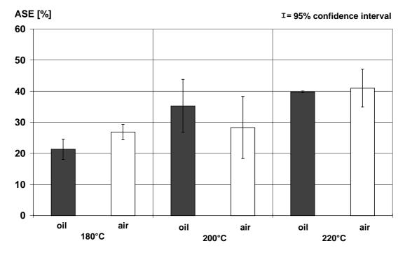
Fig. 6. ASE between 0 and 65% relative humidity of treated Pinus sylvestris L. (10x20x20 mm<sup>3</sup>), n=4
