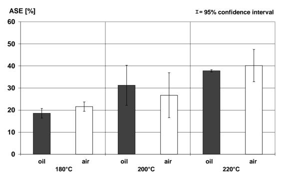
Fig. 7. ASE between 0 and 85% relative humidity of treated Pinus sylvestris L. (10x20x20 mm<sup>3</sup>), n=4
