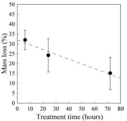
Fig. 3 Effect of treatment time on durability against the brown-rot fungus, *Fomitopsis palustris*.
