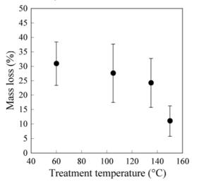
Fig. 2 Effect of treatment temperature on durability against the brown-rot fungus, *Fomitopsis palustris*.
