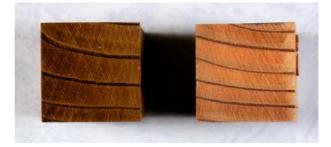
Figure 1 Photograph of the heat-treated samples Left: sample treated at 135 °C for 72 hours Right: untreated sample
