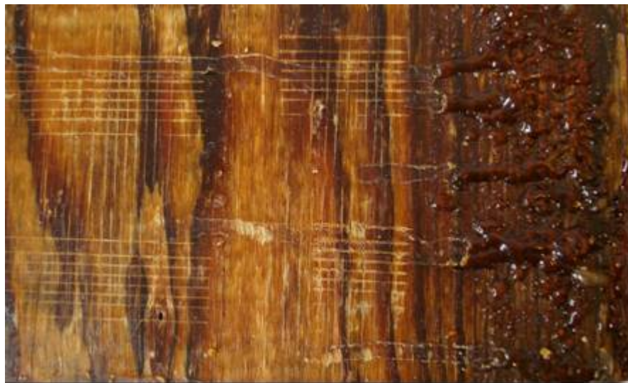
Figure 2 Oil bleeding from oil-thermal-treated pine presumably with initially intensive blue stain
