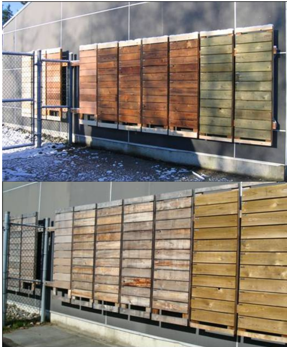
Figure 1 Appearance changes of the siding in Vancouver after 14 months
