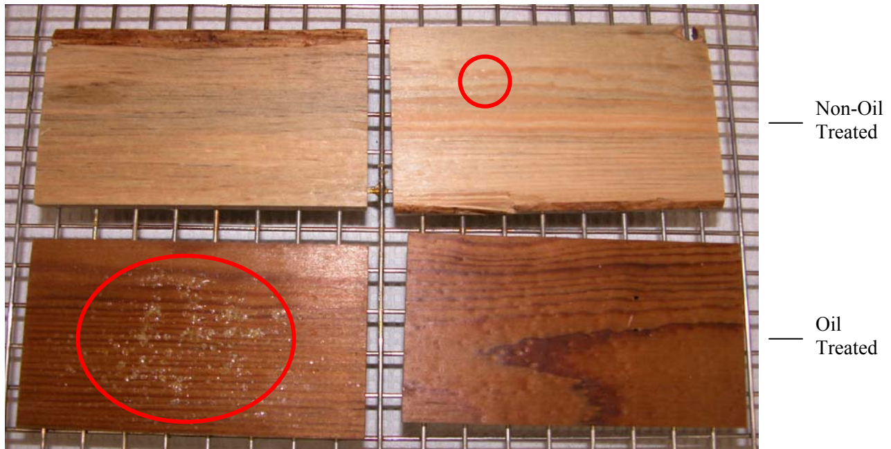
Figure 4. Adhesion of clear finishes on oil-treated and control specimens after conditioning for 6 h at 65°C, followed by 24 h at 105°C (resin beads circled in red)
