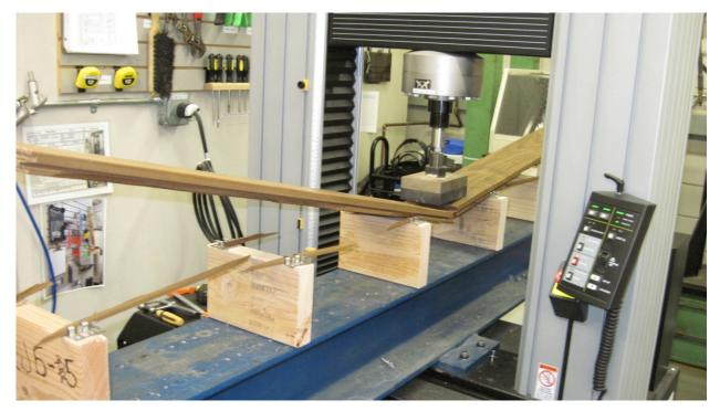
Figure 4.--Typical failure of decking when using clips. The lower tongues fail, resulting in the deck lifting significantly.
