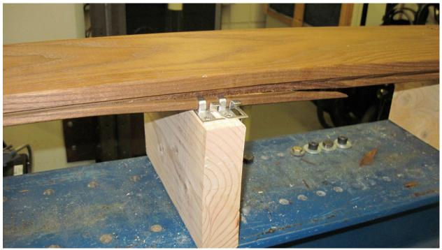
Figure 3.--Typical failure of lower tongue when decking installed with clips.
