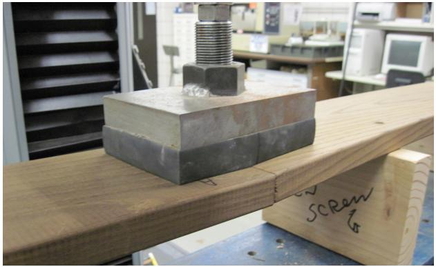
Figure 6.--Control specimen tested with butt joint at midspan.
