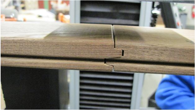
Figure 1.--End-joint tested to evaluate bending characteristics.
