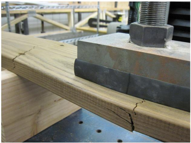
Figure 7.--Typical failure of a control sample without an end-joint under the load.
