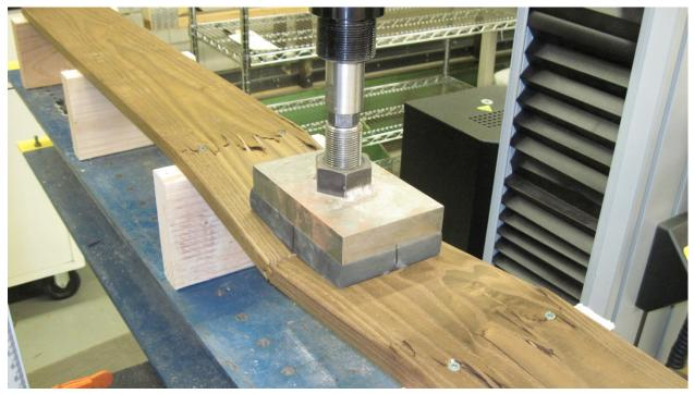
Figure 5.--Typical lumber showing failure mode. This sample was face-screwed to the joist edge.
