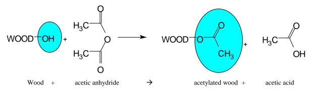
Figure 2: Acetylation: replacing OH-groups by larger and heavier CH<sub>3</sub>-groups
