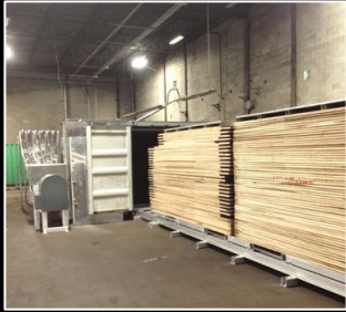
Loading lumber to the kiln
